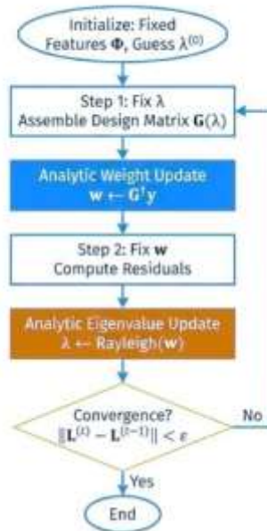
Figure 5: The flowchart displays a system which updates through pre-defined deterministic processes. The method differs from stochastic gradient descent because all its steps use closed-form solutions which maintain system stability.
